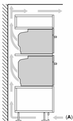
A: Dovod vazduha  $\geq 200 \text{ cm}^2$
