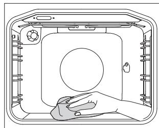
**1** Okrenite DUGME ZA IZBOR SISTEMA PEĆENJA na Aqua clean. DUGME ZA IZBOR TEMPERATURE postavite na 70°
