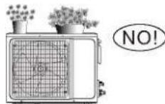
**Don't stand on the top of the outdoor unit or place heavy things on it.** This could cause personal injuries or damage the unit.
