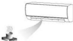
**Don't let the air conditioner blow against the heater appliance.** Otherwise it will lead to incomplete combustion, thus causing poisoning
