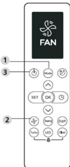
1. When push the **SWING** button, the horizontal louver changes 6 degree in angle for each push. If pushing more than 2 seconds, the louver will automatically swing up and down.
