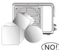
**Don't block air inlet or air outlet.** Otherwise, the cooling or heating capacity will be weakened, even cause system stop operating
