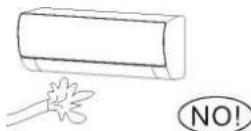
**Don't use liquid or corrosive cleaning agent wipe the air conditioner and sprinkle water or other liquid either.** Doing this may cause electric shock or damage to the unit.
