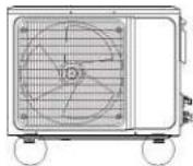
**Please note whether the installed stand is firm enough or not.** If it is damaged, it may lead to the fall of the unit and cause the injury.
