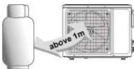
**Don't install air conditioner in a place where there is flammable gas or liquid. The distance between them should above 1m. It may cause fire even explosion.**
